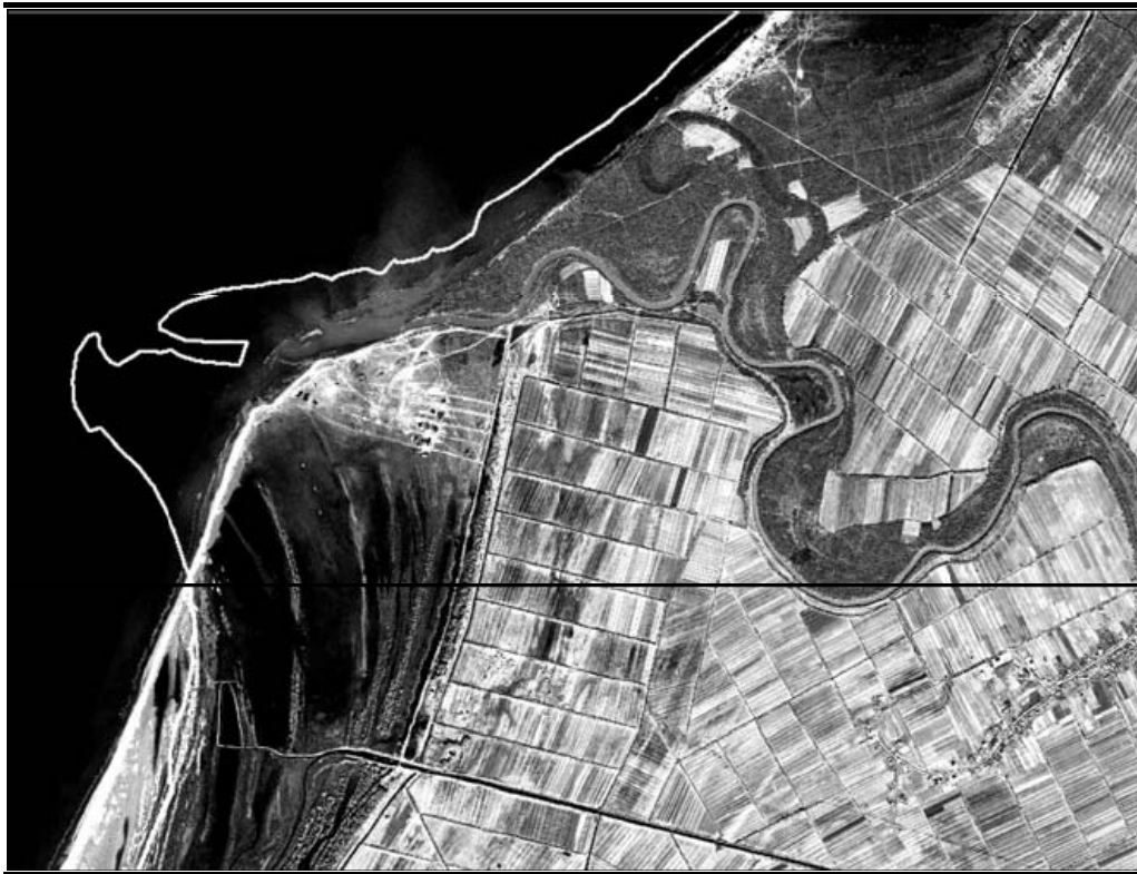
Figure 5.2.1c Coastal Erosion Movement nearby the Erzeni River Delta (white line represents the previous coast line)
