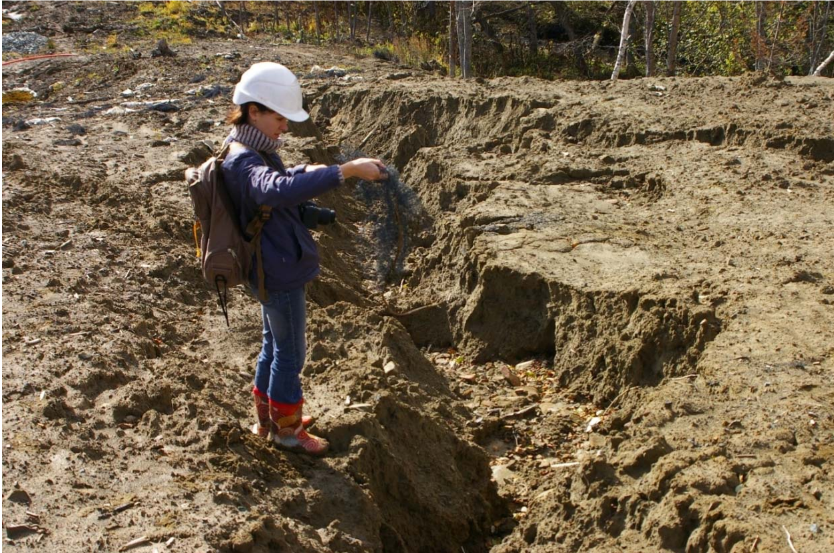
October 23, 2007: KP 491.3. Left bank of the Krutoyarka River. Galya is holding the remains of failed enkamats. Though a very few anti-erosion measures such as this were observed, they absolutely failed to achieve their intended purpose.
