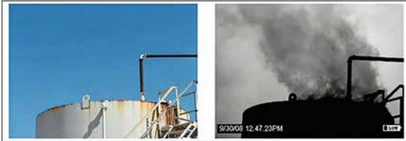
The photo on the left depicting an element of a compressor station was taken using an ordinary camera, while the photo on the right depicting the same element was taken using an infrared camera. We can see leakages of volatile organic compounds.
