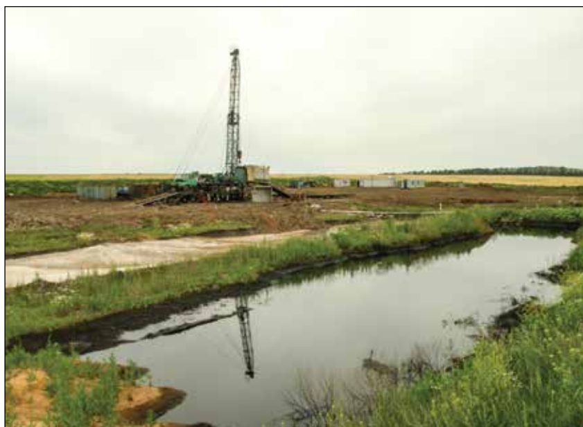
The sump for drilled solids at the well No. 17 owned by Ukrgasvydobuvannia company in the Kamianska area (village of Yaremivka, Kharkiv region), 2013. Photo: Oleh Savvitskyi
