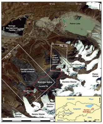
The company's 2015 technical report<sup>11</sup> adds: "Thawing of the moraine dam, to an extent that it allows for piping or overtopping of the dam, may lead to a dam breach and the uncontrolled release of lake water that can potentially erode a section of the tailings dam and damage other downstream facilities."
