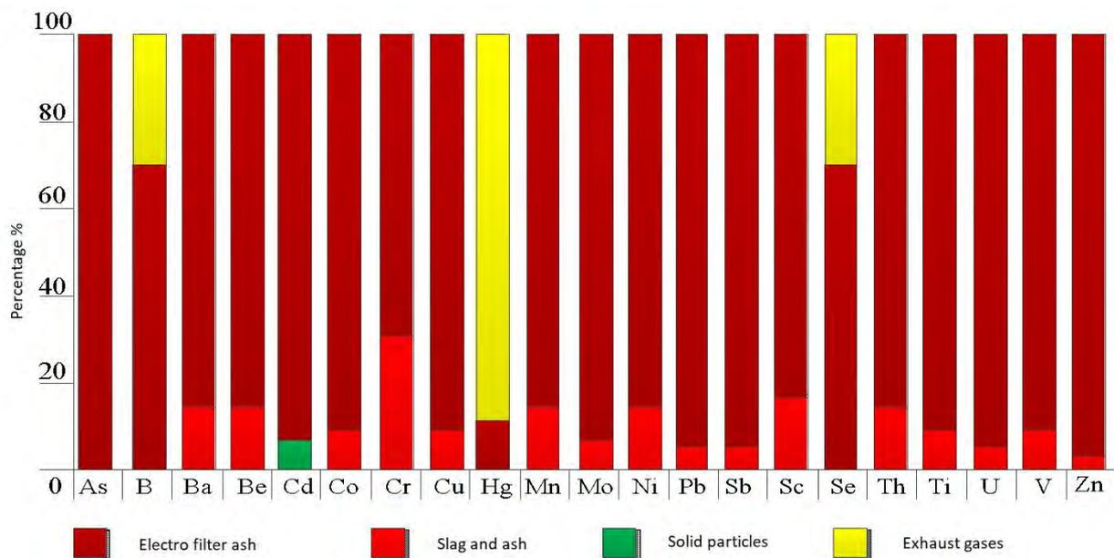
**Figure 3.1.** Distribution of some heavy metals in electro-filter ash and slag, solid particles and exhaust gases<sup>7</sup>
