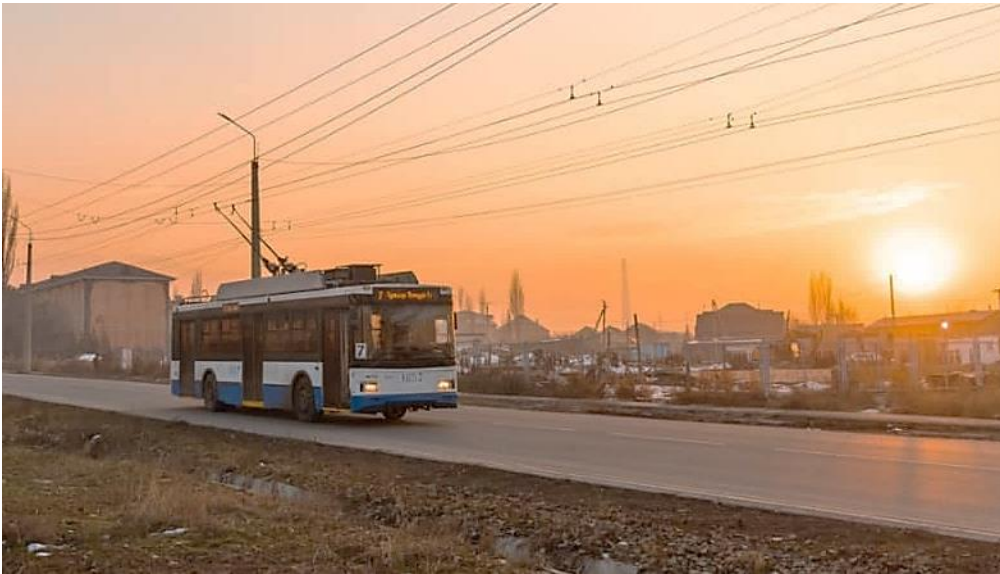
A Bishkek trolleybus powered by electricity from dual overhead wires. Photo: Save Bishkek's Trolleybuses initiative
